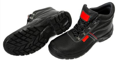
Safety footwear is defined by standard HRN EN ISO 20345:2012 which as the basic requirement (SB) posts the toe cap resistance 200 J (TC 200 J), resistance to fuel oils (FO) and slip resistance (SR).
